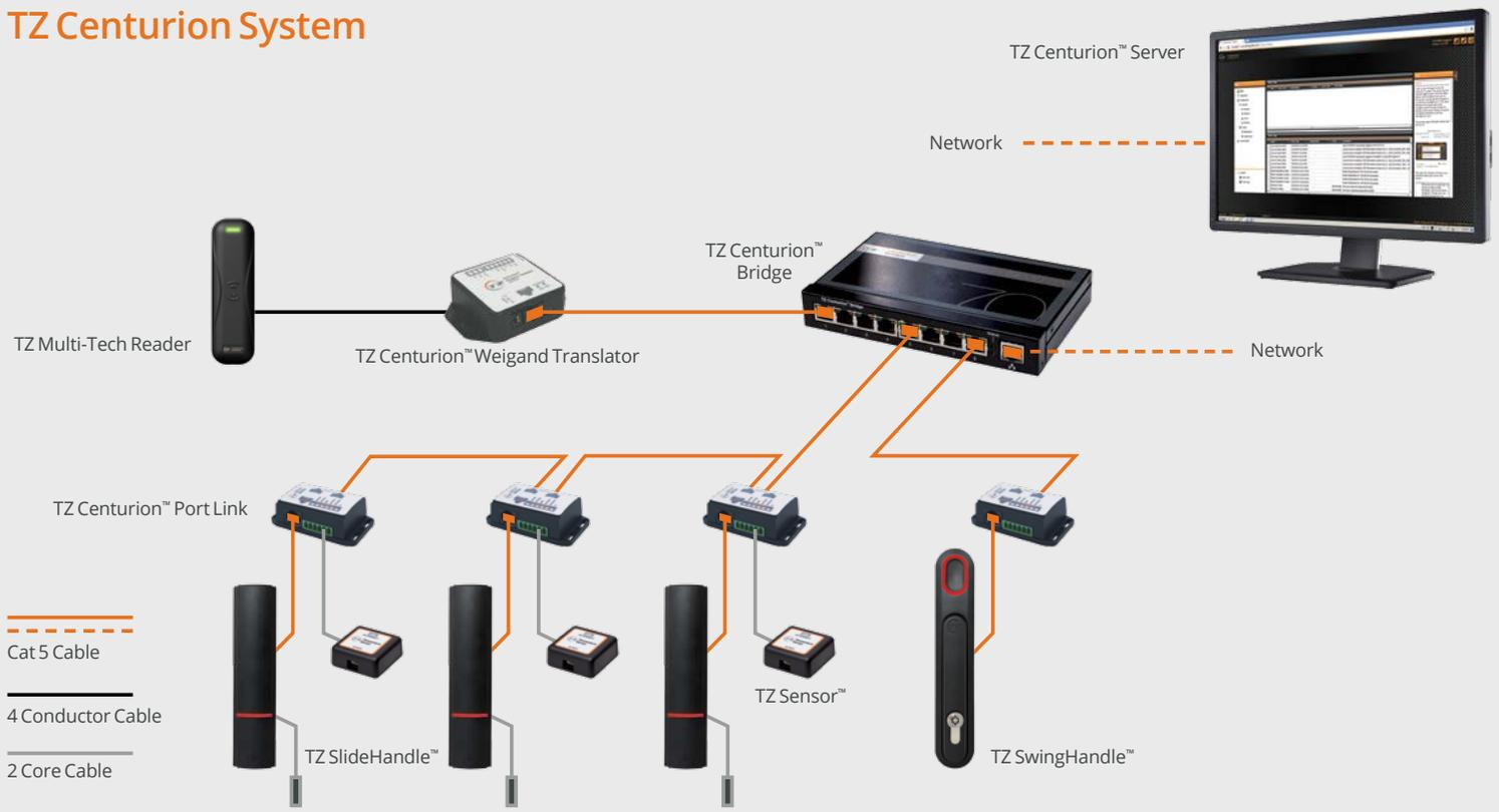
LES chose to install the TZ Centurion System throughout the new data center because the System easily meets and even exceeds the level of protection that LES Corporate Security demanded for cabinet level micro-security.
